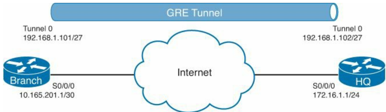
Figure 31-1. GRE Tunnel Configuration
