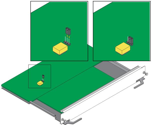
As shown in the figure above pins 1 and 2 must be connected on jumper block J31, which is located near the lithium battery, to ensure a successful FPGA upgrade. (Please note that pin 1 is located the closest to the front panel, pin 2 is in the middle, and pin 3 is located closest to the backplane connector.) If pins 1 and 2 are not connected as shown in the figure above then perform the steps described in "Program Enable Jumpers Not Installed" on page 38 to perform an FPGA upgrade.
