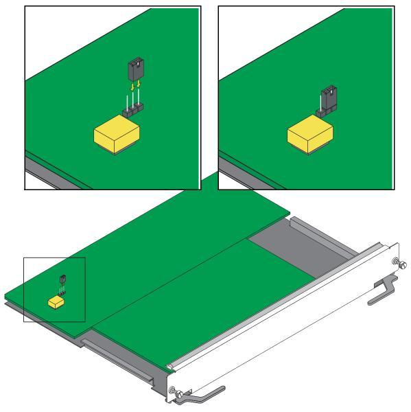
As shown in the figure above pins 1 and 2 must be connected on jumper block J21, which is located near the lithium battery, to ensure a successful FPGA upgrade. (Please note that pin 1 is located facing the bottom edge of the CMM, pin 2 is in the middle, and pin 3 is located the closest to the top edge of the CMM.) If pins 1 and 2 are not connected as shown in the figure above then perform the steps described in "Program Enable Jumpers Not Installed" on page 38 to perform an FPGA upgrade.
